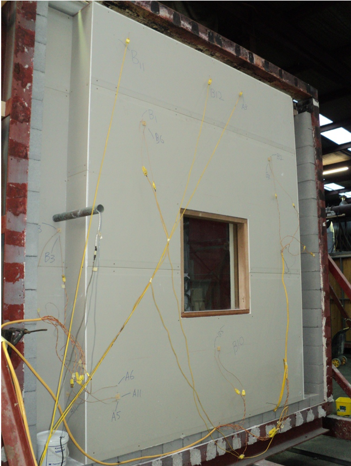
Figure A6.3 Unexposed face of test specimen at completion of test.
