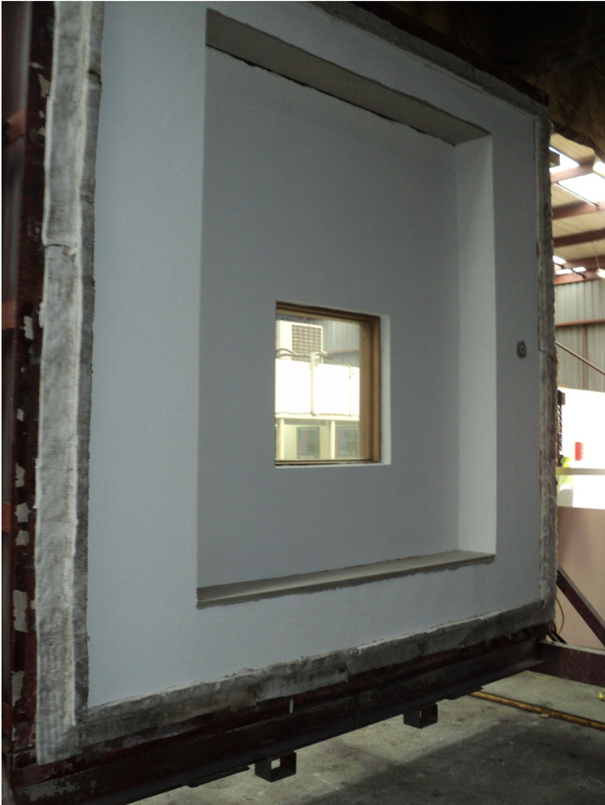
Figure A6.2 Exposed face of the specimen prior to the test.
